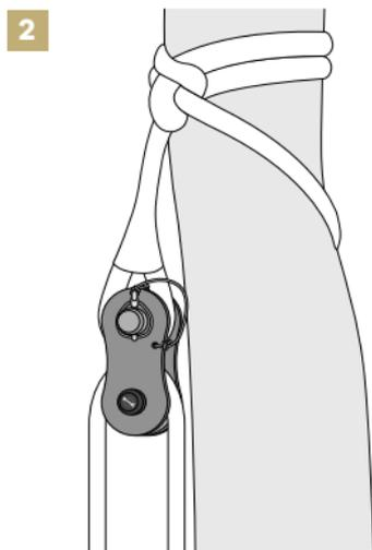
Remove the safety linchpin, slide the upper axle and open the swinging cheek plate. Place the rigging rope in the sheave's groove, place a textile sling (or strap) around the upper axle. Close the swinging cheek plate and the upper axle, lock in place with the safety linchpin. Check to make sure the ring is engaged in the safety catch.
